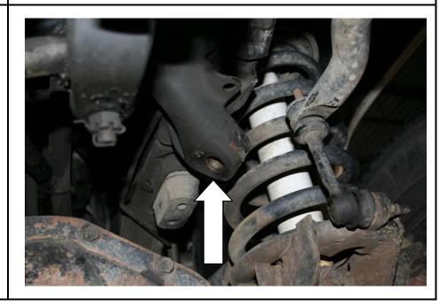
Clean the outside frame rail where the retrofit bracket will mount.
