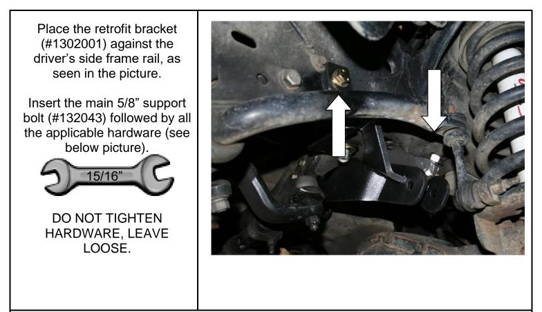
\* You will only need to use the second 1302044 washer if the weld line is very large on the driver's side factory track bar mounting face.
