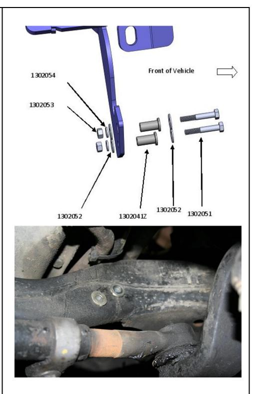
Now using the remaining <sup>1</sup>/<sub>2</sub>" x 5" bolt to secure the last bracket point.
